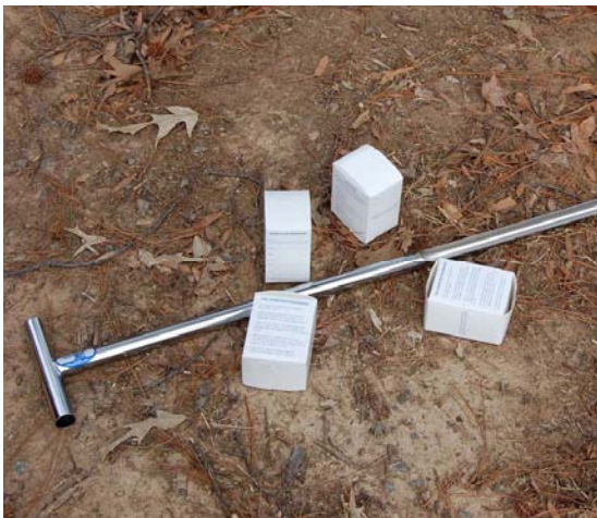
Soil sample boxes and a device that pulls up soil cores. (U of Arkansas System Division of Agriculture file photo by Leo Espinoza)
